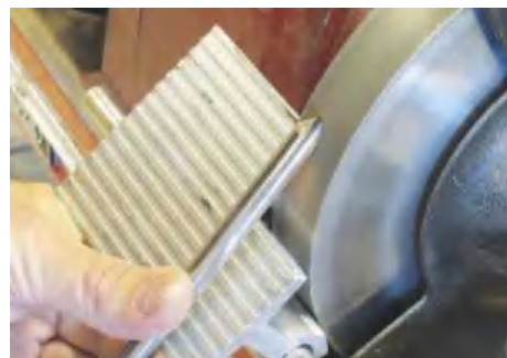
▲ Pic.3 Rotate the tool against the grindstone. As you near the side you need to slide the tool up the wheel, as shown here; this will put the required fingernail profile on the tool
